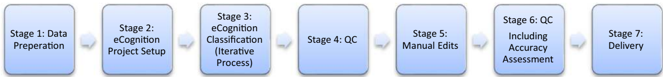
Fig. 2 Habitat Mapping Workflow. This shows the 7 stages in the Habitat Mapping process, ranging from Data Preparation to Delivery. There are two stages covering eCognition, then stages 4, 5 & 6 which cover the QC and Manual Edits which help to ensure a high quality mapping product
