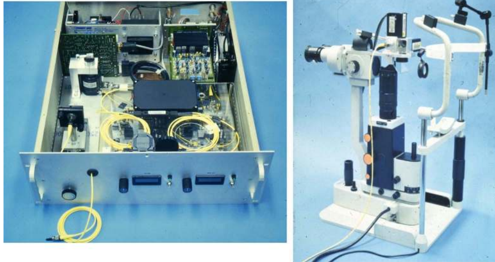
FIGURE 6. The first OCT retinal imaging prototype instrument was designed by (EAS) at MIT Lincoln Laboratory in 1993. The imaging engine was reduced in size from a 1-m 2 lab table to a compact and robust 19-inch wide unit. High speed A-scanning at 160 mm/s enabled rapid acquisition of retinal images. The patient interface was designed around a slit-lamp biomicroscope. The OCT beam is scanned using a pair of galvanometer actuated mirrors. This system was designed for use at the NEEC and imaged several thousand patients during the mid-1990s. Image courtesy of Eric Swanson.
