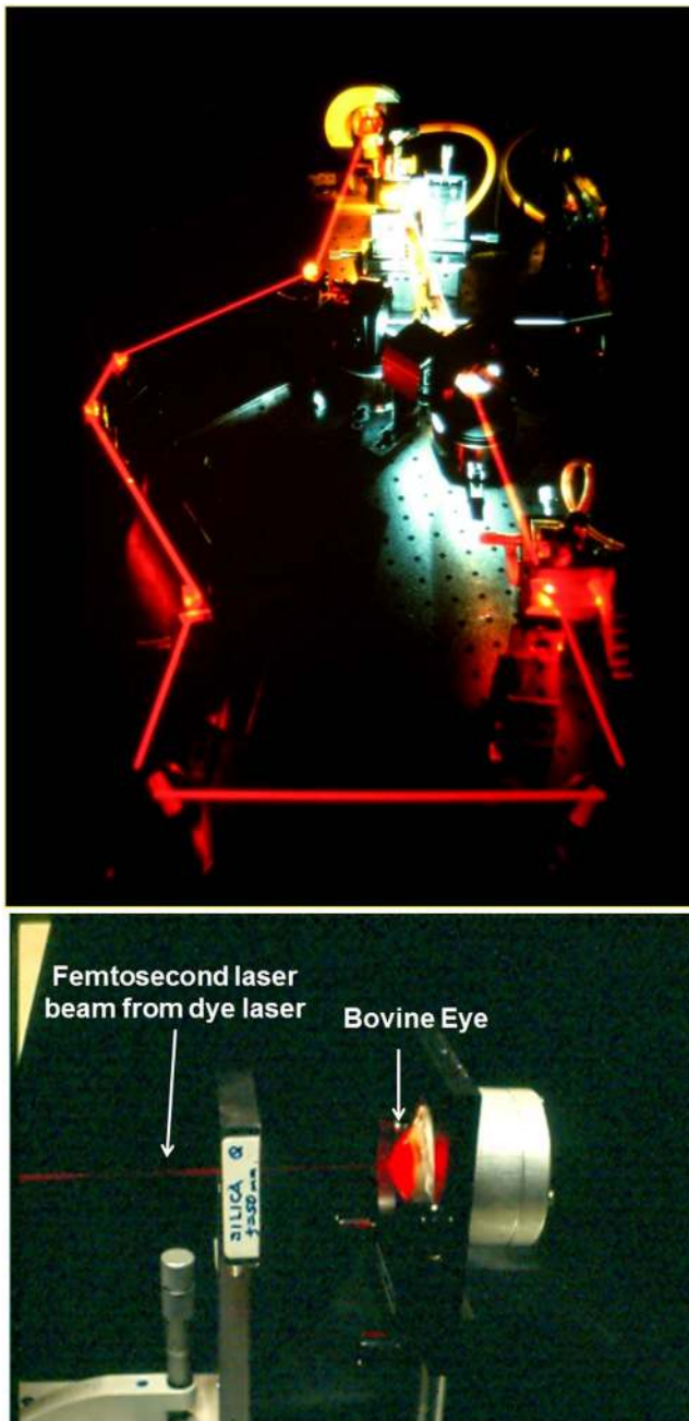
FIGURE 2. (Top) The colliding pulse femtosecond dye laser was state of the art in the 1980s and could generate record pulse durations of less than 100 fs. This technology enabled fundamental studies of ultrafast phenomena in physics, chemistry, and photobiology. We began to explore biomedical applications at MIT in the mid-1980s. (Bottom) Early experiment measuring femtosecond light echoes in an ex vivo bovine eye.
