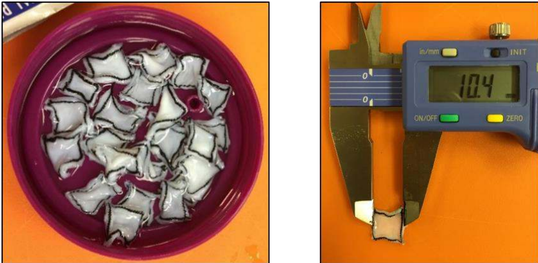
Figure 22: (Left) Representative 22 3-layer AF patches in a specimen lid. (Right) One 3-layer AF patch 10.4 mm in width.
