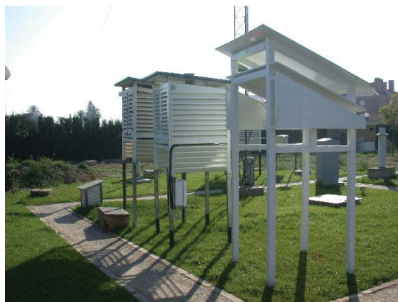
Figure 3. Picture showing both the old Montsouris stand and the new Stevenson screen as replicated in the Meteorological Garden of Murcia (Courtesy of the project SCREEN). This figure is available in colour online at www.interscience.wiley.com/ijoc
