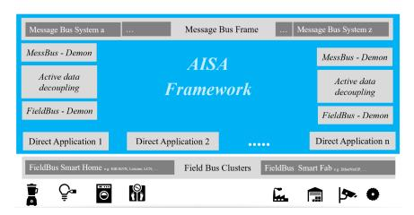
Figure 21. Overview of the AISA communication architecture (own elaboration).
