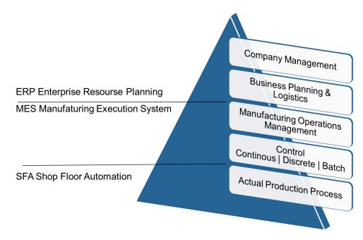
Figure 20. Functional hierarchy according to ISA95 (own elaboration).
