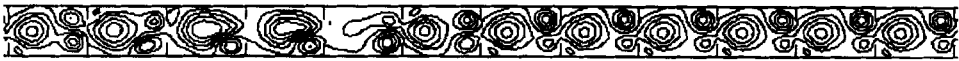
FIGURE 22. A plot of instantaneous streamlines in the (x, y) -plane for a fully developed, asymmetric sinusoidal flow at the point of flow reversal ( t = \text{an integer} ). A two-dimensional numerical simulation was used to obtain the streamfunction distribution, with the spatial periodicity relaxed to twelve cells, as depicted. The flow was started from rest with a small perturbation to allow differences in the flow in each cell to develop. Re and St were 200 and 1.0 respectively. Streamfunction \psi is plotted at intervals of 0.1. The flow is periodic over one oscillation cycle, but it is clear from the figure that the flow is not spatially periodic over each cell of the geometry.
