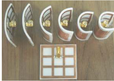
Figure 8. Curved antennas with different central angle \alpha ( 0^\circ , 45^\circ , 90^\circ , 135^\circ , 180^\circ , 225^\circ and 270^\circ ) for experiment.
