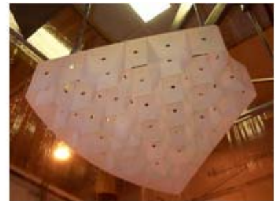
Figure 2 - Abrasive Waterjet (AWJ) cutting of mirror cores reduced the mass of lightweight mirrors. By segmenting the mirror core, the cost and schedule risk of a catastrophic failure in AWJ was also reduced.
