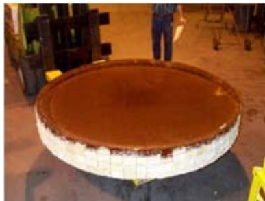
Figure 2 - Abrasive Waterjet (AWJ) cutting of mirror cores reduced the mass of lightweight mirrors. By segmenting the mirror core, the cost and schedule risk of a catastrophic failure in AWJ was also reduced.
