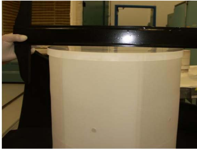
Figure 6 - The demonstration mirror was slumped to a 2.5m radius of curvature to allow center of curvature optical testing in the Marshall Space Flight Center chamber.
