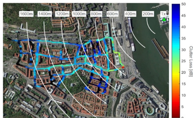
Fig. 5. Clutter loss measured at 28 GHz in Gothenburg. The transmitter (basestation) location is marked with Tx.
