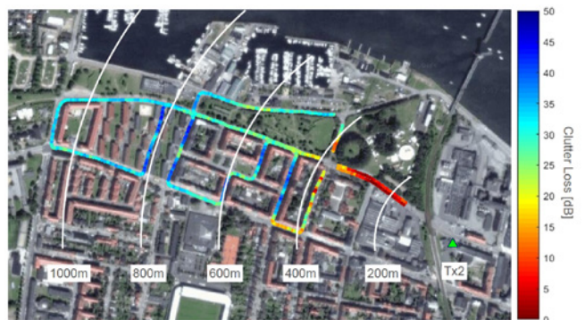
Fig. 3. Clutter loss measured at 18 GHz for the base station location Tx2 in Aalborg.
