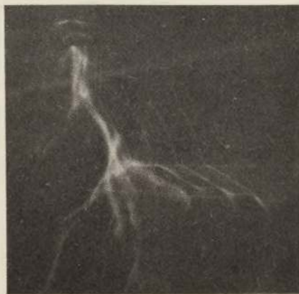
FIG. 23. Positive point electrode: earthed plane electrode. R=100,000 ; P=5 .
