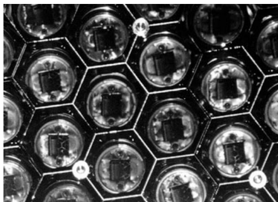
Figure 39. PMTs and rhodium-plated light-catchers in the SOB.
