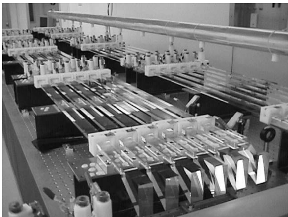
Figure 29. A bar assembly station showing a set of six bars with wedges already attached.
