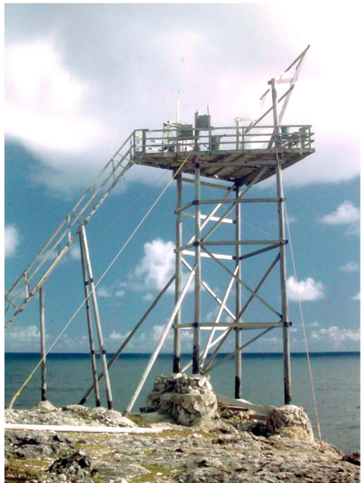
Fig. 2. African dust sampling tower, on the coast at Cole's Pasture, Saint Philip, Barbados (13.1547109°N, 59.421748°W). Parkin et al. named the facility "Öpik Tower" to honor Ernst Öpik, the Estonian astronomer and astrophysicist who had done much research on meteors, most notably on the entry of high-speed bodies into the atmosphere and their consequent ablation. Dust is collected on nylon mesh screens that were suspended from the crossbars at the front of the tower, which faces to the east, into the trade winds. See Figs. ES2 and ES3 for other images related to tower activities.
