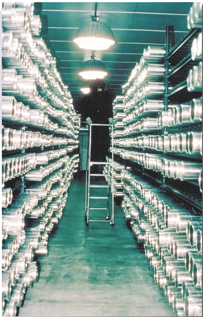
Figure 5. Three kilometers of ice stored as a gleaming library of cylinders in the US National Ice Core Laboratory in Denver, Colorado. Analysis of the ice, drilled from the Greenland icecap during the 1990s, provided a compelling record of precipitous climate changes around the end of the last glacial epoch. The findings stimulated computer simulations of the atmosphere–ocean–ice system; those simulations suggested that such changes could befall us within the next few hundred years. (Photo by Kendrick Taylor, DRI, University of Nevada, Reno, courtesy of the National Oceanic and Atmospheric Administration Paleoclimatology Program/US Department of Commerce.)
