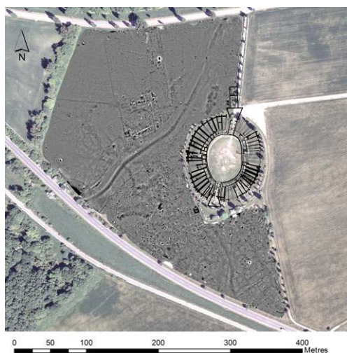
Figure 5. Magnetogram of the western area around the municipal amphitheatre showing the remains of the gladiatorial school and its surroundings. The prominent winding linear feature indicates a ditch dug for the installation of an aqueduct. As the building complex clearly respects this ditch, it is assumed to predate the construction of the gladiatorial school. An extended refuse dump obvious in the magnetic and radar data at the southern corner of the building proves that the ditch in Roman times was a distinct depression separating the gladiatorial school from the surrounding area of the amphitheatre (graphics: Wolfgang Neubauer and Alois Hinterleitner).
