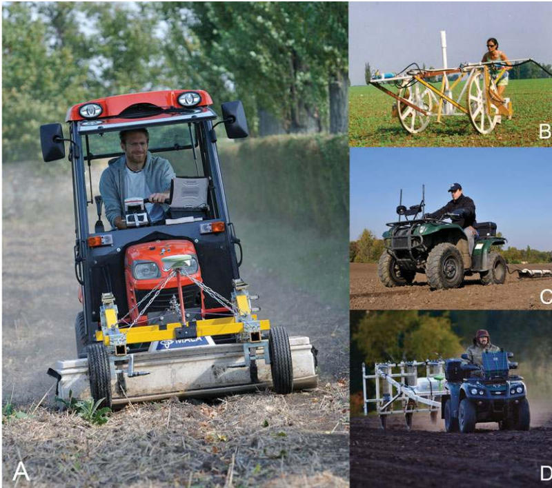
Figure 4. Geophysical measurement systems used in the detection of the gladiatorial school at Carnuntum: A) the MALÅ Imaging Radar Array (MIRA) with 16 \times 400\text{MHz} channels spaced at 8cm. The RTK-GPS receiver is situated centrally above the GPR antenna box. The system is hydraulically mounted in front of a small tractor; B) PICODAS MEP750 Caesium magnetometer with five sensors (sensitivity 0.001\text{nT} ) manually operated with optoelectronic distance measurement; C) motorised dual EM-21S sensor with four coils; D) motorised 10-sensor Foerster fluxgate gradiometer array operated behind a quad ATV (photos: Geert Verhoeven and Wolfgang Neubauer).
