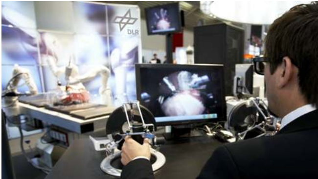
Fig. 3. The DLR MiroSurge robotic system for surgery. Depiction of the minimally invasive robotic surgery scenario. In the foreground: input console with force reflecting input devices (left and right hand, cp. Sec. IV) and 3D vision. In the background: slave unit with three MIRO robots (cp. Fig. 2).
