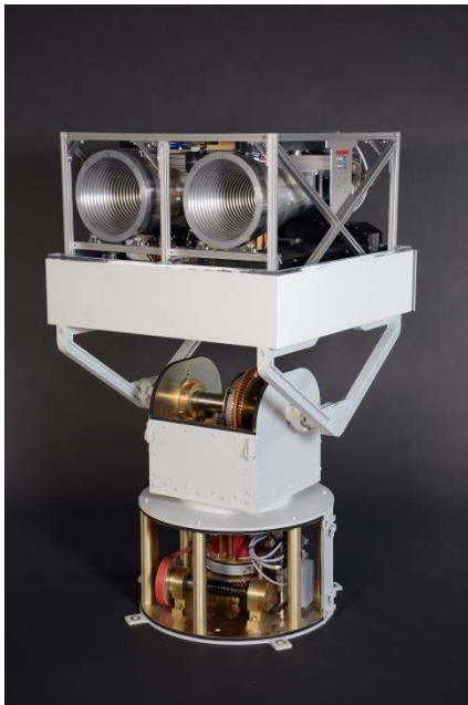
2 Figure 3 C-band remote-controlled 'Kalibri' transponder, housing of the positioner removed.
