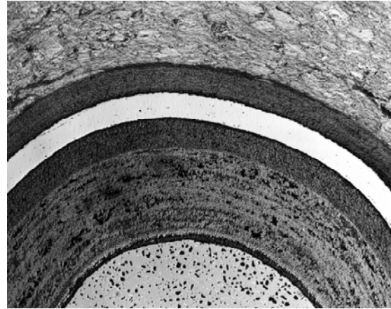
Figure 13. Photomicrograph of German AVR fuel after irradiation.
