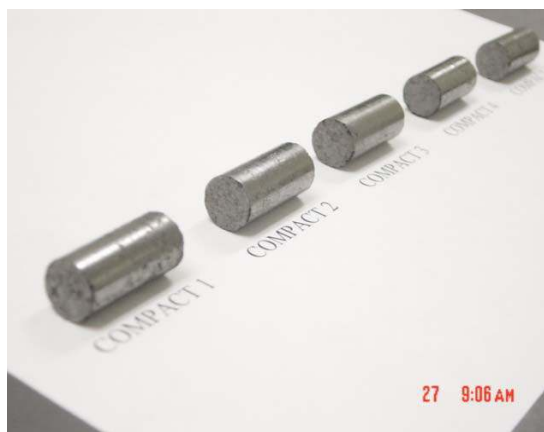
Figure 8. Compacts produced using ORNL thermosetting resin process.
