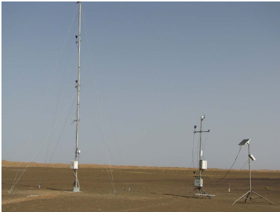
889 890 Figure 20: Meteorological station deployed in the Sahara desert for the study of dust lifting process 891 and its feedback on the electrical properties of the atmosphere.
