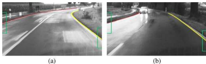
Fig. 12. (a) Entering a sharp turn in s05 at t = 200 . (b) Too-short detected lanes (with the left lane shown in black and the right lane in white).
