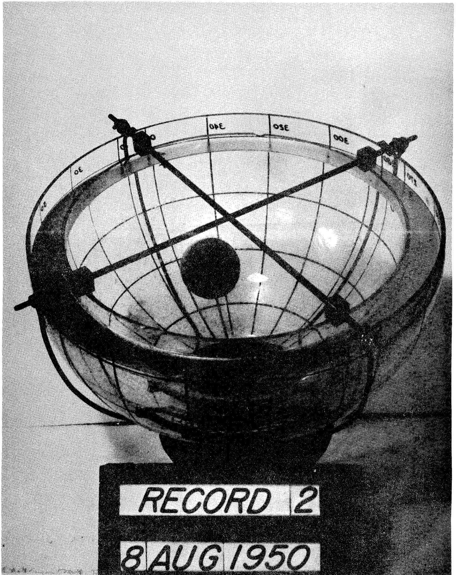
Fig. 1: The rotating hemispherical shells for studying two-dimensional motions of homogeneous fluid around an obstacle used by Fultz, Long and Frenzen.
