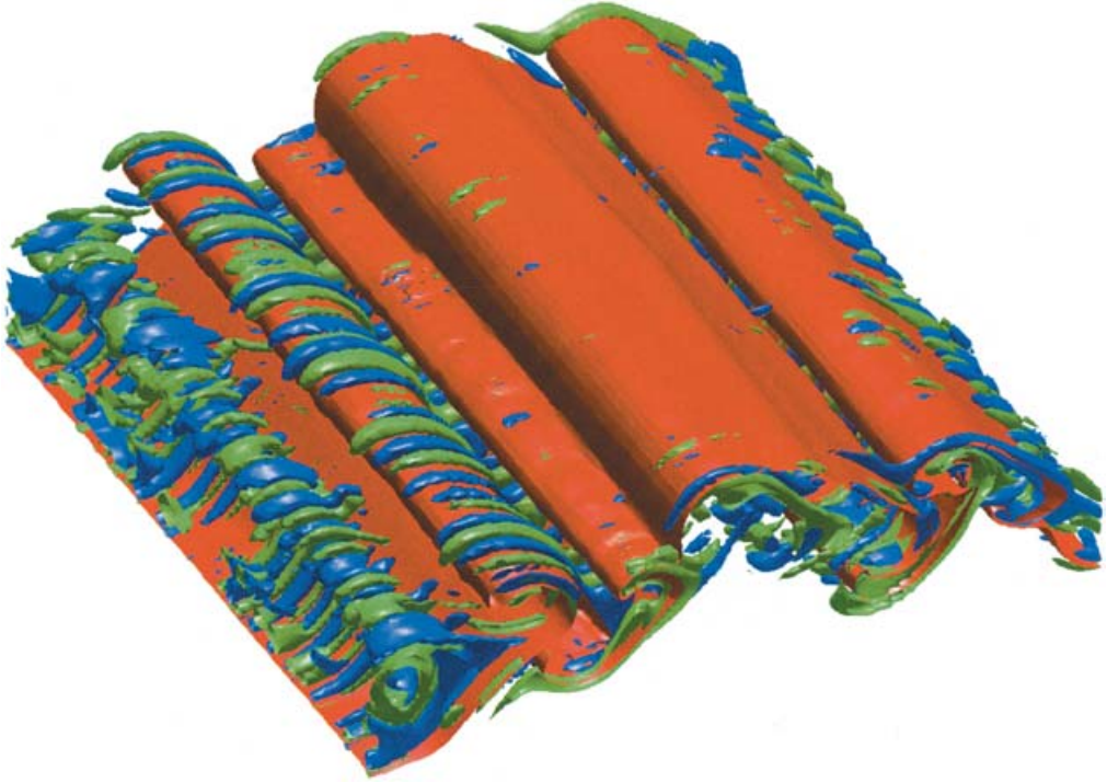
FIGURE 17. Isosurfaces of \rho=0 (red) and longitudinal vorticity \omega_1 for a breaking interfacial wave with interface thickness k\delta = \pi/10 , corresponding to regime A in figure 10, when the cross-stream kinetic energy is maximized at t/T = 2.33 after release of forcing. Blue and green isosurfaces represent positive and negative longitudinal vorticity of magnitude \omega_1/\omega = 1/2 . The wave propagates from left to right.
