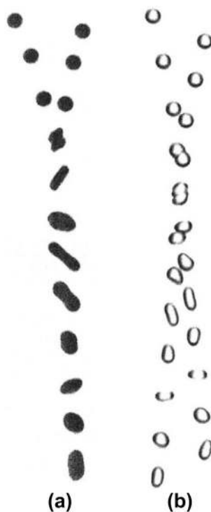
Fig. 15 Droplet collision for milk concentrates and glycerol solution at similar conditions: a We = 19 , B = 0.38 , Oh = 0.022 for coalescence of milk 20% and b We = 18.1 , B = 0.4 , Oh = 0.021 for bouncing 40 vol% glycerol
