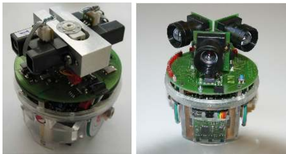
Fig. 5. Two “top” extensions for the e-puck robot: an infrared distance scanner (left) and a large field of view linear camera (right).
