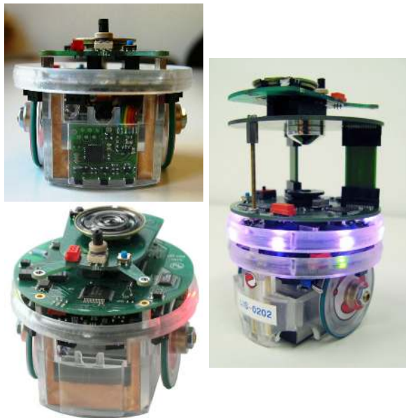
Fig. 6. Left top: A bottom extension to measure the ground color. Left bottom: a “sandwich” extension implementing a Zigbee radio link. Right: A complete visual communication system consisting of two “sandwich” extensions.
