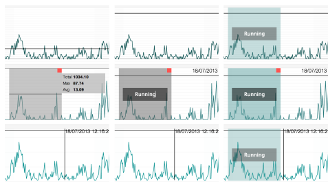
Figure 2: A screenshot of the labelling feature in use. First the user shift-clicks (or pinches) to create an interval. They then double tap to bring up a text label and type their label. When they press enter, the interval label is created for all data sources at that time period.
