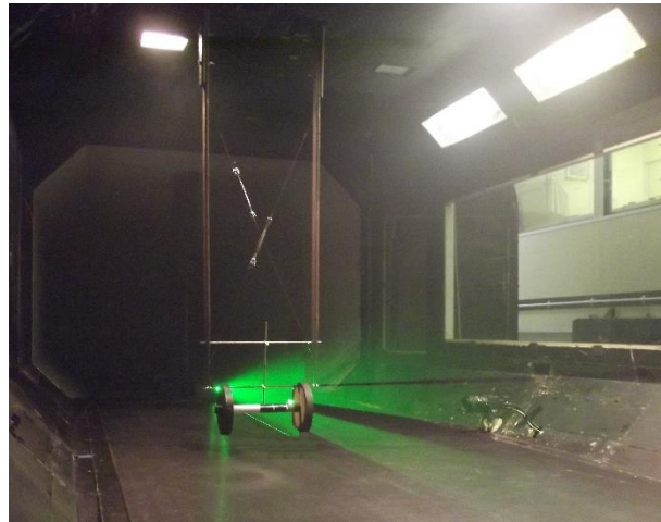
Figure 1. Front view of the PIV experimental setup of isolated wheelset case
