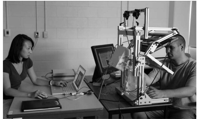
Fig. 1. Simulator setup. Upper panel : Conceptual design of the tool used in the experiment. Lower panel : Photo of the actual tools used in the experiment. The observer (left) sits opposite the trainee (right) and can monitor the insertion visually. The side of the phantom facing the trainee is covered to prevent the trainee from direct visual access to the target.
