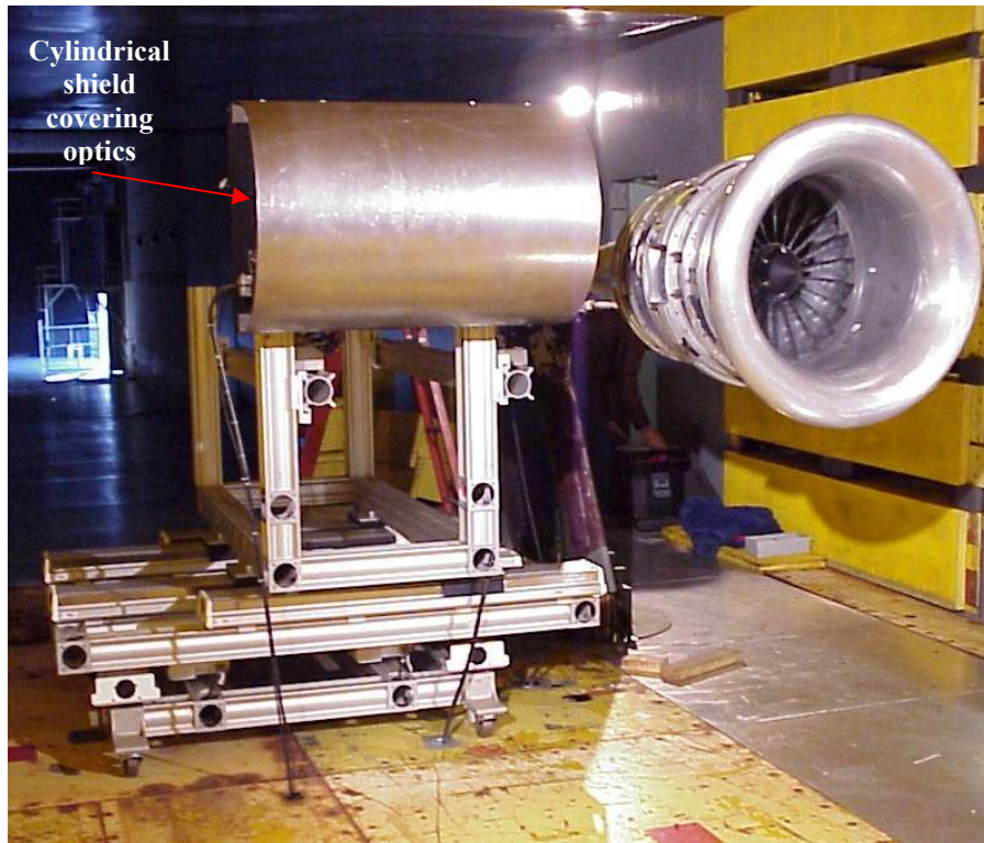
a) LDV system hardware installed next to the research fan model in the wind tunnel
