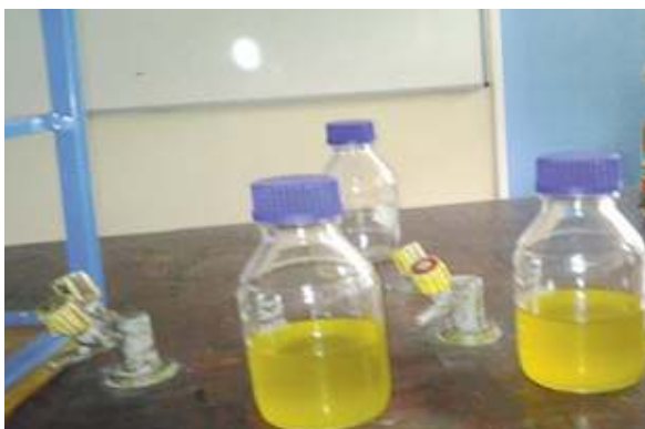
Figure 2: The distillate samples from the waste plastic pyrolysis oil samples.
