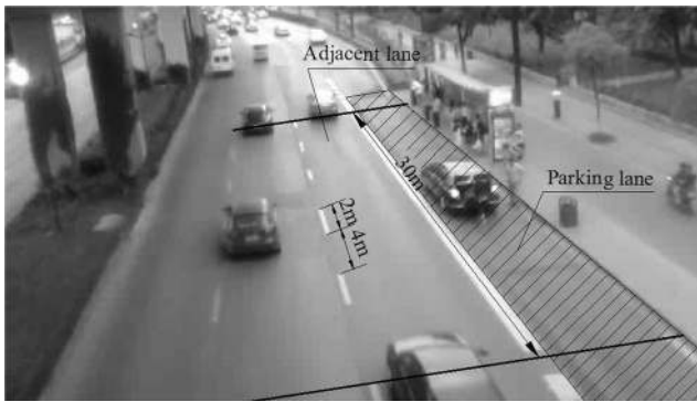
Fig. 9 The measuring method of traffic density
