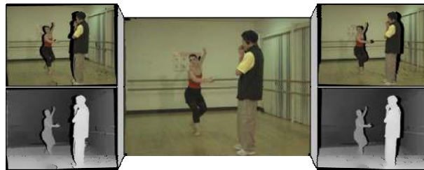
Fig. 5. Rendering of a virtual intermediate view from the projected MVD data of two neighboring original cameras.
