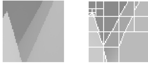
Fig. 2. Example of a quadtree decomposition. Each block, i.e. node, of the quadtree is approximated by one modeling function.
