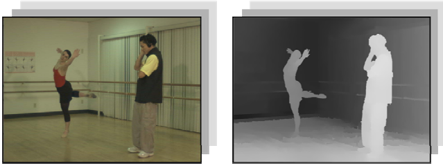
Fig. 1. Example for the MVD format with texture image (left) and corresponding depth-image (right).
