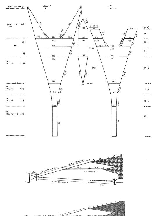
Fig. 1. Standard survey bottom trawl. Rigging with 40 m and 20 m sweeps.
