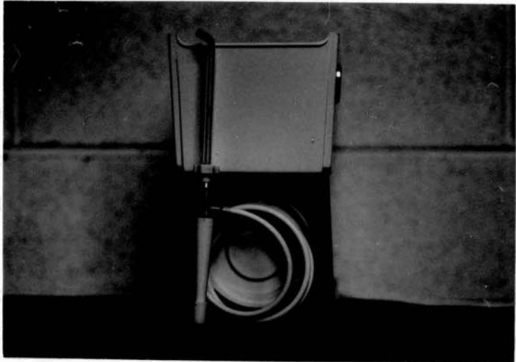
FIG. VI FORCED ORAL LAVAGE UNIT USED IN EXPERIMENT
