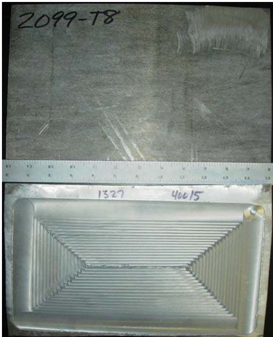
Figure 2-1. As Received (AR) and Friction Stir Processed (FSP) plate provided along with composition by weight percent of AF/C458
