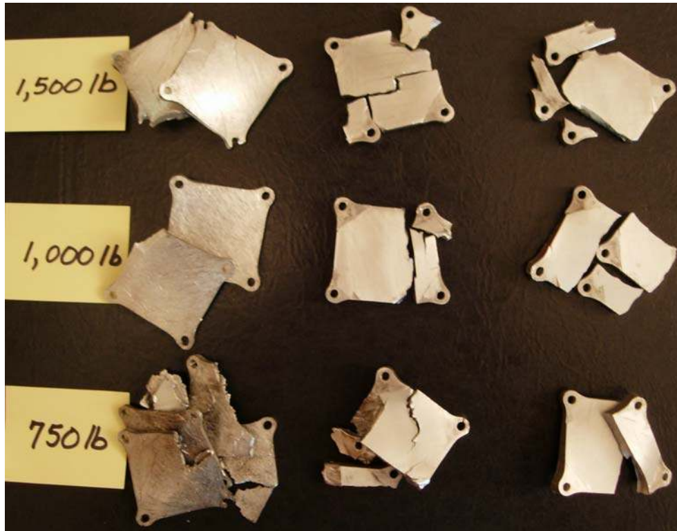
Photograph of anticlastic test specimens after failure @ various loads. From left to right, AR, FSP, and FSP+HT plate
