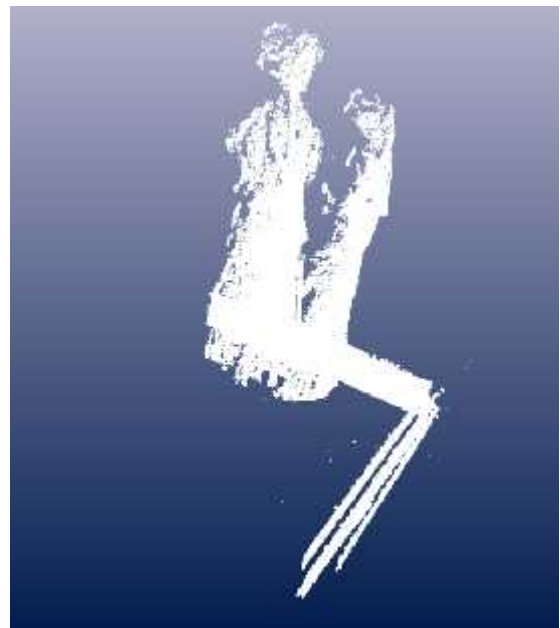
Figure 9. Gross errors of point cloud obtained from %50 compressed images by SURF.
