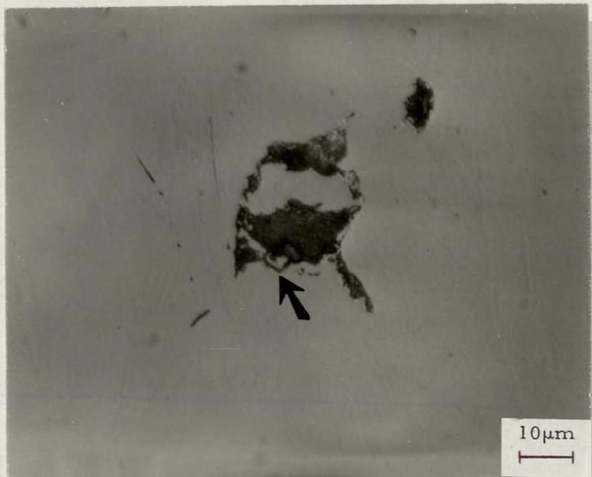
Figure 20 Optical micrograph of a sectioned tensile specimen of the 2070 \text{ MN/m}^2 (300 ksi) material strained to 0.487. The Ti(C,N) inclusion nucleation site is marked by an arrow. The tensile axis is vertical.
