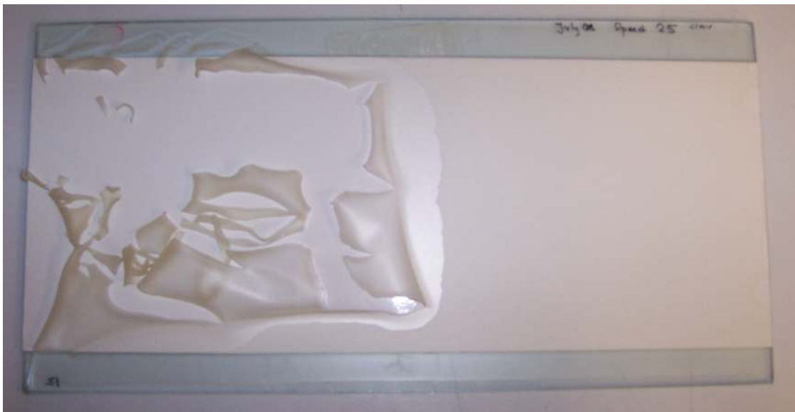
Figure 15: Film cracking due to low casting speed
