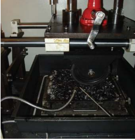
FIGURE 6: Internal part illustration for wheel rutting tester.
