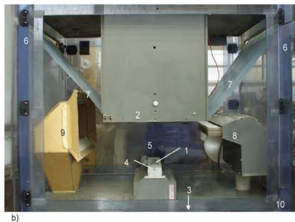
Figure 1. Electrospinning setup used to collect nanofibers on the surface of reinforcing materials. 1: rotary electrode, 2: grounded plate electrode, 3: high-voltage power supply, 4: polymer solution, 5: fiber formation space, 6: rollers, 7: moving belt collector, 8: air inlet, 9: air outlet, 10: chamber.
