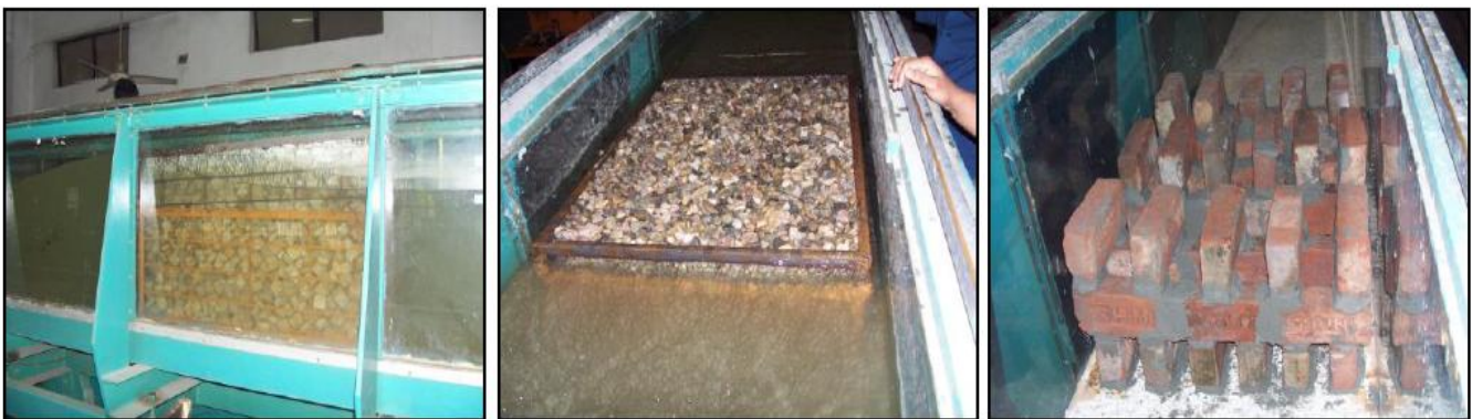
Fig. 1. Breakwater made of (a) randomly placed c.c. block, (b) stone chips and (c) brick framework.
