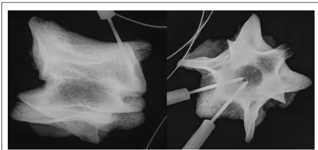
FIGURE 1 | Radiograph showing the location of the temperature probes within the vertebra in a lateral (left) and axial (right) view.
