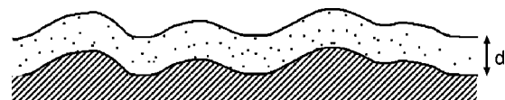
FIG. 5. The adhesion interaction pulls the elastic slab into complete contact with the rough substrate surface.
