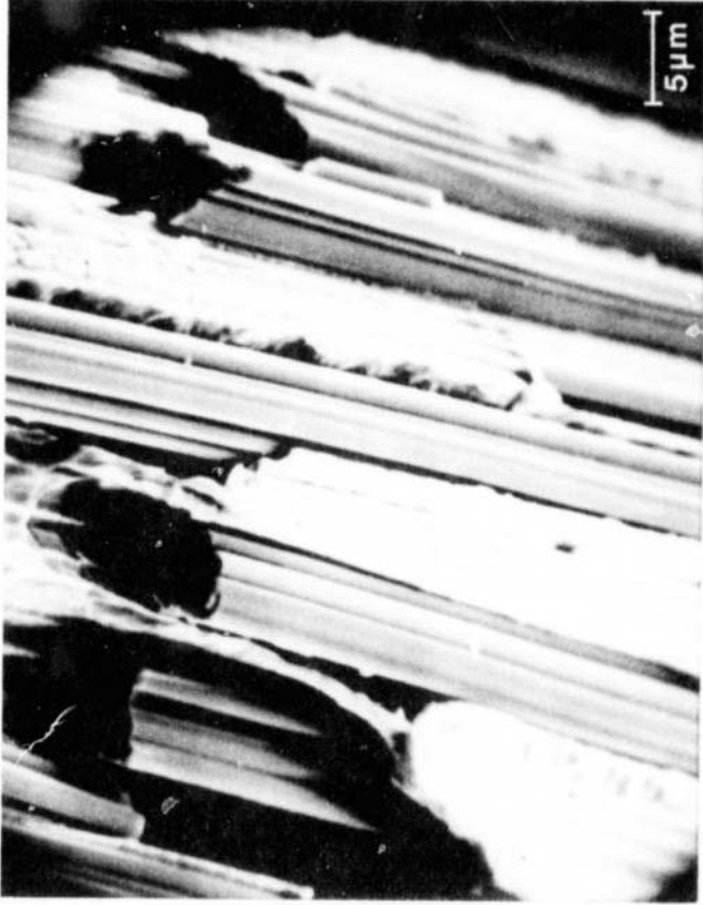
Fig. 9 - Scanning electron micrograph of the fracture surface of a transverse Al-Gr composite specimen.
