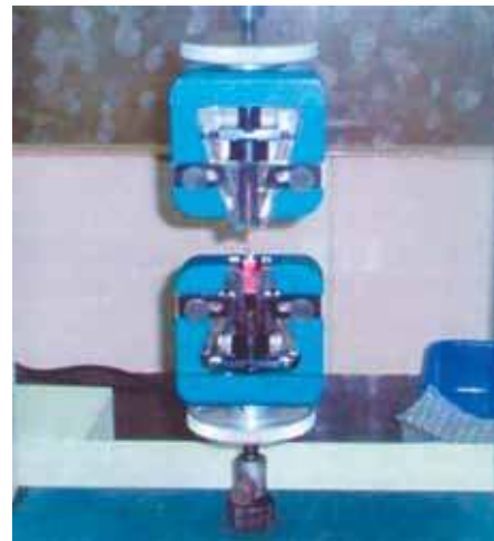
Fig. 6: Testing a sample in Hounsfield universal testing machine
