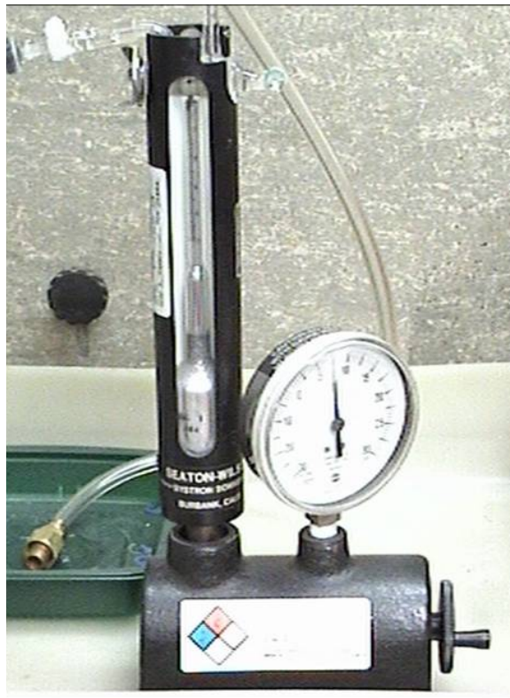
Figure E.8: Aire-ometer used for measuring air content percentage.
