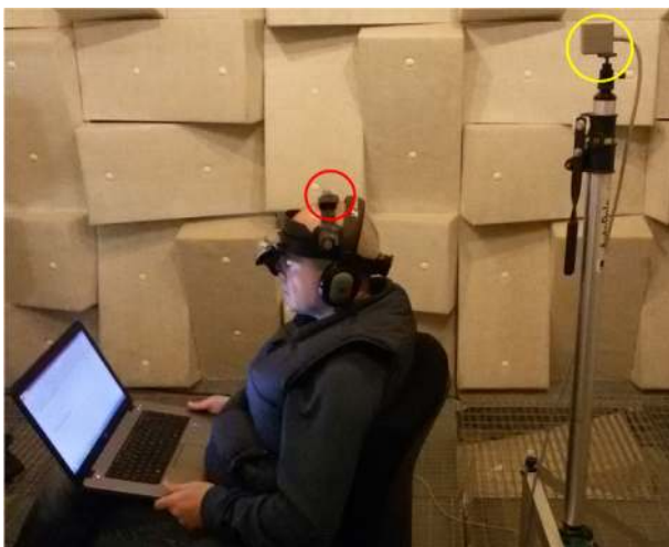
Fig. 5—A picture of the IVR experimental set-up with the head-mounted motion sensor (red circle) and the motion tracker (yellow circle).
