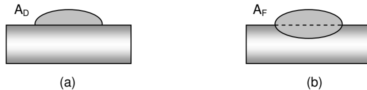
Figure 2. 15 Schematic illustration showing the definition of (a) deposited and (b) fused weld metals.
