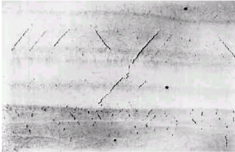
Figure 3. 8 A photograph of a typical pattern of chevron cracking in a longitudinal section revealing 45° angle with the plane of the plates in a butt joint (after http://www.twi.co.uk ).
