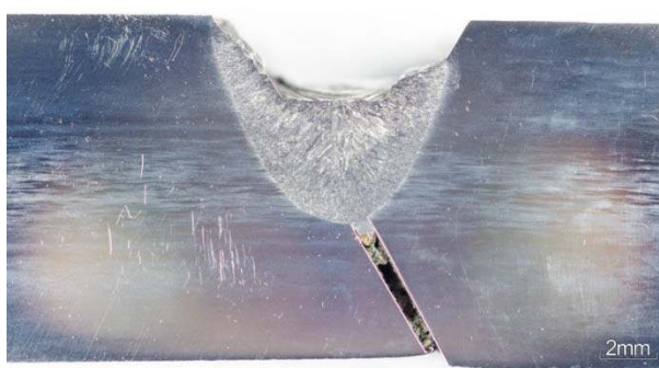
Fig. 2. Tekken sample W1. Welding bead performed underwater with heat input 1.1 kJ/mm. No imperfections. Beracha's etch.
