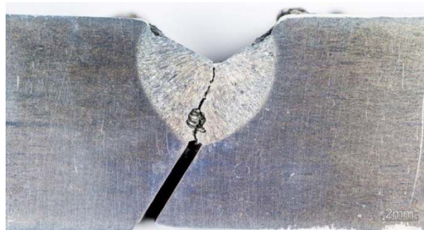
Fig. 5. Tekken sample W4. Welding bead performed underwater with heat input 3.0 kJ/mm. Crack in the weld. Beracha's etch.
