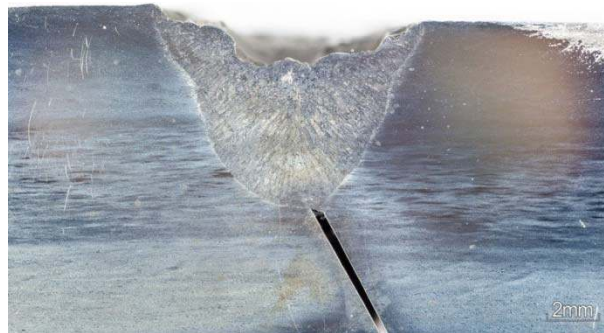
Fig. 4. Tekken sample W3. Welding bead performed underwater with heat input 3.0 kJ/mm. No imperfections. Beracha's etch.
