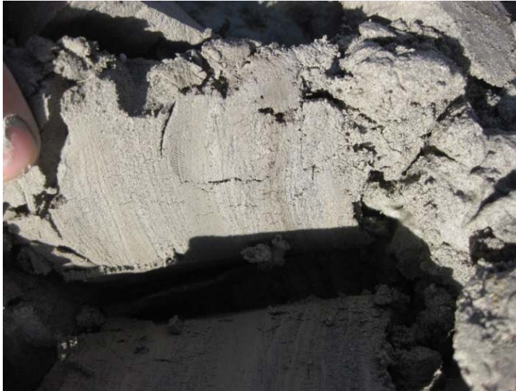
Figure 8. Fine sand sample with thin silty laminae from test field SF/SU1 (see Fig. 7).
