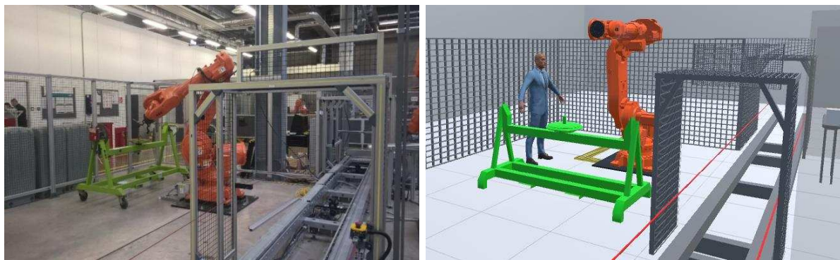
(ii) Workshop environment replicated in Unity. The human manikin is used as a visual aid to understand the reaction of users during playbacks.
