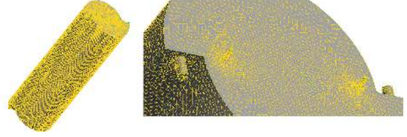
FIGURE 3: Schematic diagram of the computational domain of asymmetric vortex chamber.
